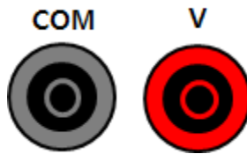
Voltage Input Terminal
